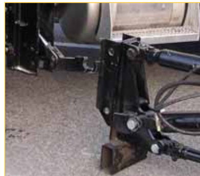
Model L1925HYD wing portion (hydraulically detachable coupler)
